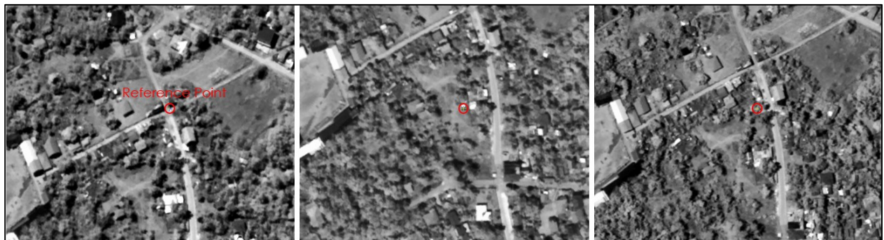
Figure 6: Raw Level 10 tri-stereo KOMPSAT-3 images shown with a reference point to assess georeferencing quality.
